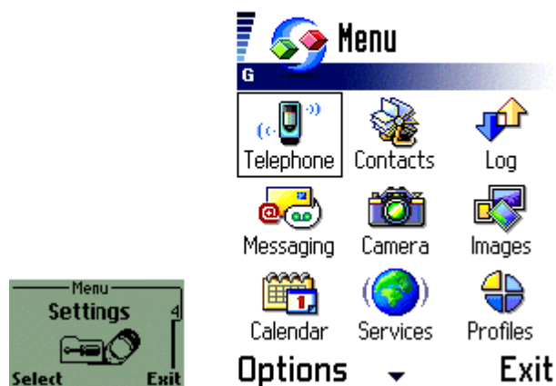
Figure 1. On the left a monochrome display of the Nokia 6210 mobile phone with a resolution of 96x60 pixels. On the right the display of the Nokia 7650, featuring 4096 colours and a resolution of 176x208 pixels.
