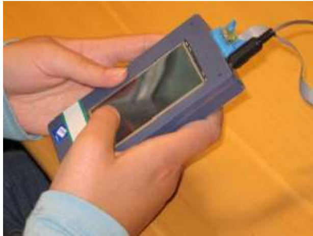
Fig. 23. Users were holding the device with their both hands and pressed the virtual buttons with their other hand's thumb.
