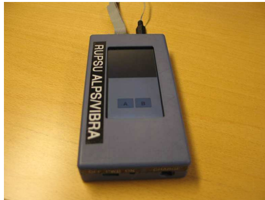
Fig. 18. Touchscreen device enhanced with tactile feedback.
