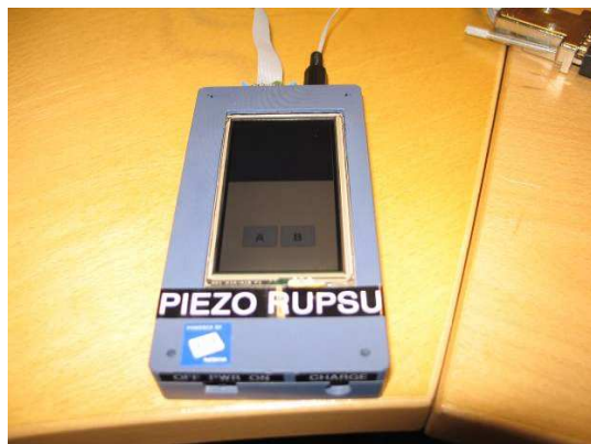
Fig. 12. Touchscreen device enhanced with tactile feedback.
