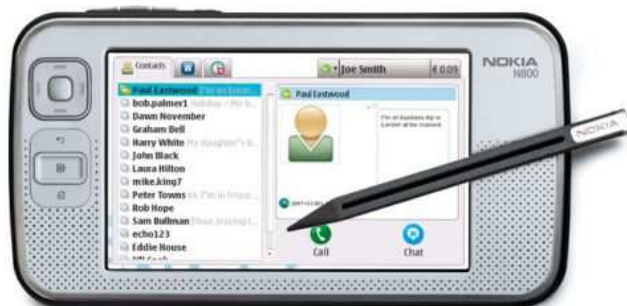
Fig. 1. The Nokia N800 Internet Tablet, a touchscreen device, which uses a stylus for interaction.
