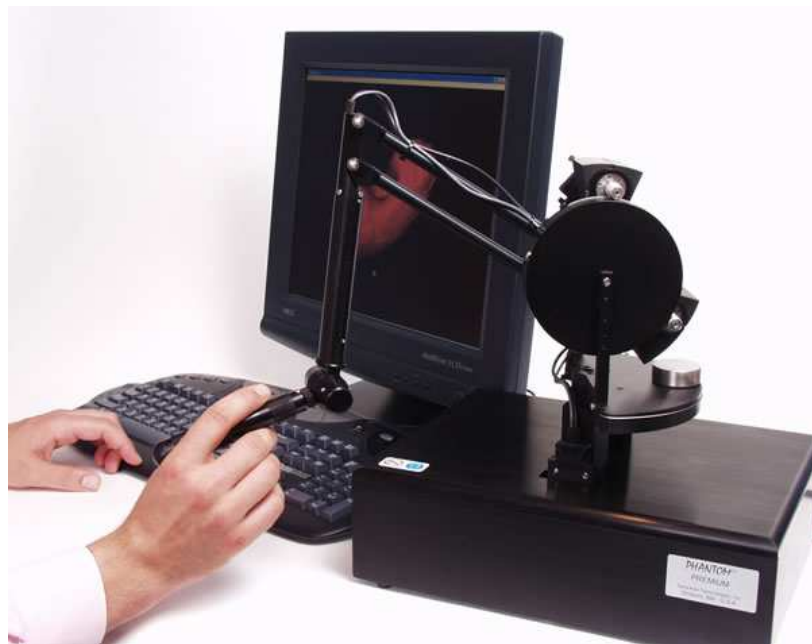
Fig. 7. The PHANTOM haptic device by SensAble technologies.
