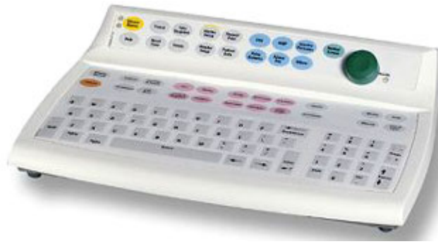
Figure 7 The Datex-Ohmeda anesthesia record keeper keyboard for patient monitors includes all the same function keys as the patient monitor, special anesthesia-related function keys, qwerty-keyboard keys, numeric pad and the control wheel.
