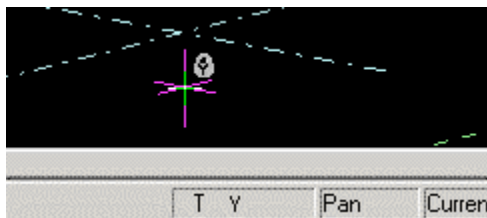
Figure 23: The axis lock symbol in the cursor. In this case the user has activated the Y -axis lock.
