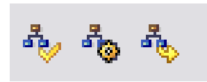
Figure 6: Shortcuts to model validation, BPEL generation (including WSDL and PXE compilation) and server deployment available in top menu.
